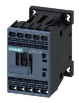
power contactor, AC-3e/AC-3, 12 A, 5.5 kW / 400 V, 3-pole, 24 V DC, auxiliary contacts: 1 NC, spring-loaded terminal, size: S00  $\,$
