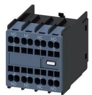
auxiliary switch, on the front, 2 NO + 2 NC, .3/.4, .1/.2, .1/.2, .3/.4, current path: 1 NO, 1 NC, 1 NC, 1 NO, spring-loaded terminal, for contactors 3RT2 and contactor relays 3RH2
