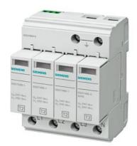
Surge arrester Type 2 Requirement class C, UC 350V Pluggable protective modules 4-pole, 3+1 circuit for TN-S and TT systems
