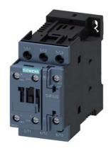
power contactor, AC-3e/AC-3, 12 A, 5.5 kW / 400 V, 3-pole, 24 V DC, auxiliary contacts: 1 NO + 1 NC, screw terminal, size: S0  $\,$
