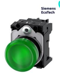
Indicator lights, 22 mm, round, metal, shiny, green, lens, smooth, with holder, LED module with integrated LED 24 V AC/DC, screw terminal
