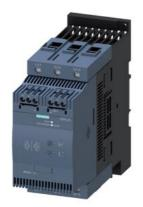
SIRIUS soft starter S3 80 A, 45 kW/400 V, 40 °C 200-480 V AC, 110-230 V AC/DC Screw terminals
