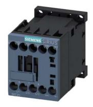
power contactor, AC-3e/AC-3, 7 A, 3 kW / 400 V, 3-pole, 24 V DC, auxiliary contacts: 1 NC, screw terminal, size: S00  $\,$
