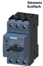
Circuit breaker size S0 for motor protection, CLASS 10 A-release 2.8...4 A N release 52 A screw terminal Standard switching capacity
