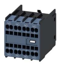
auxiliary switch, on the front, 4 NO, .3/.4, .3/.4, .3/.4, .3/.4, current path: 1 NO, 1 NO, 1 NO, 1 NO, 5 NO, 1 NO, 5 spring-loaded terminal, for contactors 3RT2 and contactor relays 3RH2
