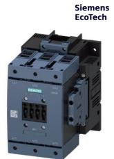
power contactor, AC-3e/AC-3 115 A, 55 kW / 400 V, AC (50-60 Hz) / DC Uc: 23-26 V 3-pole, auxiliary contacts 2 NO + 2 NC drive: conventional main circuit: box terminal control and auxiliary circuit: screw terminal
