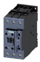
power contactor, AC-3e/AC-3, 80 A, 37 kW / 400 V, 3-pole, 24 V DC, 0.8-1.2\* Us, with integrated varistor, auxiliary contacts: 1 NO + 1 NC, screw terminal, size: S2, suitable for PLC outputs
