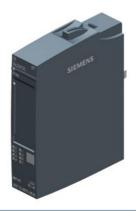
SIMATIC ET 200SP, Digital input module, DI 8x 24V DC Standard, type 3 (IEC 61131), sink input, (PNP, P-reading), Packing unit: 1 piece, fits to BU-type A0, Colour Code CC01, input delay time 0,05..20ms, module diagnostics for: short-circuit of sensor supply, wire break, supply voltage
