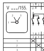
X Kontakt geschlossen/contact closed    X Kontakt geschlossen ohne Unterbrechung/contact closed without interruption
