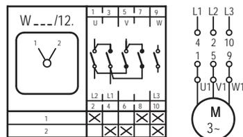
X Kontakt geschlossen/contact closed    X Kontakt geschlossen ohne Unterbrechung/contact closed without interruption
