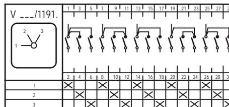
X Kontakt geschlossen/contact closed    X Kontakt geschlossen ohne Unterbrechung/contact closed without interruption
