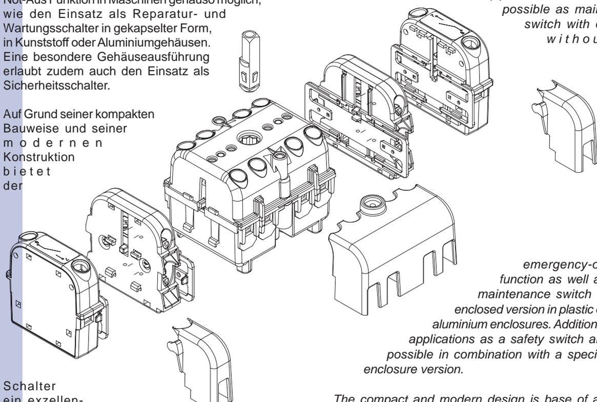
*emergency-off function as well as maintenance switch in enclosed version in plastic or aluminium enclosures. Additional applications as a safety switch are possible in combination with a special enclosure version.*
