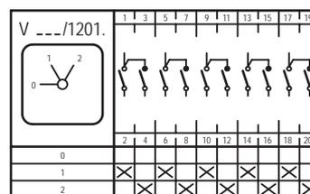
X Kontakt geschlossen/contact closed    X Kontakt geschlossen ohne Unterbrechung/contact closed without interruption
