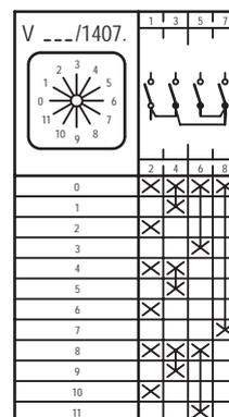
X Kontakt geschlossen/contact closed    X Kontakt geschlossen ohne Unterbrechung/contact closed without interruption
