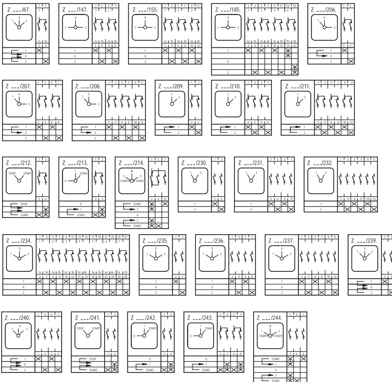
X Kontakt geschlossen/contact closed    X Kontakt geschlossen ohne Unterbrechung/contact closed without interruption
