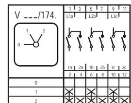
X Kontakt geschlossen/contact closed    X Kontakt geschlossen ohne Unterbrechung/contact closed without interruption
