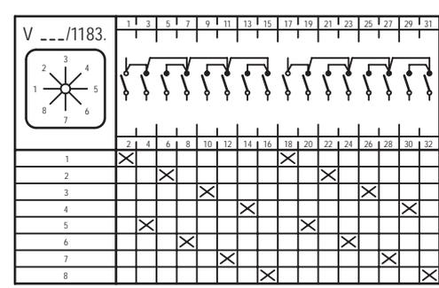
X Kontakt geschlossen/contact closed    X Kontakt geschlossen ohne Unterbrechung/contact closed without interruption
