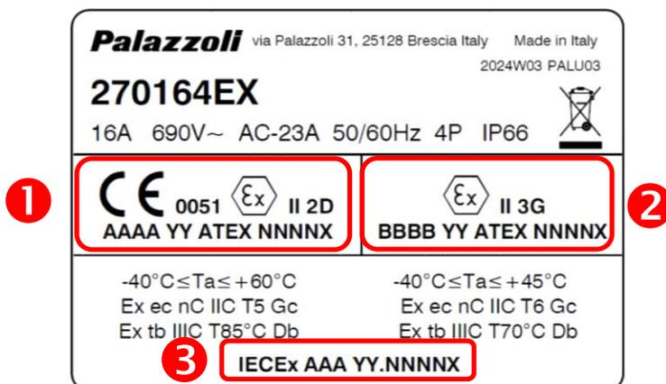
**1** - Marking related to the equipment classified in Group II Category 2D, the presence of the CE marking with the number of the Notified Body shows the application of Module D (Annex IV of the ATEX Directive), quality assurance of the production process. The certificate number "AAAA YY ATEX NNNNX" shows the application of the mandatory Module B (Annex III of the ATEX Directive), EU-type examination.
